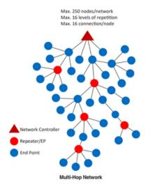
G.hn Spirit Grid software supports a large-scale, multihop network of up to 250 nodes in a single network domain. Spirit Grid's self-organize-network (SON) feature enables autonomous device installation and configuration, optimal signal path selection, and network self-healing capabilities.
