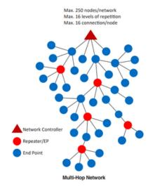
G.hn Spirit Grid software supports a large-scale, multi-hop network of up to 250 nodes in a single network domain. Spirit Grid's self-organize-network (SON) feature enables autonomous device installation and configuration, optimal signal path selection, and network self-healing capabilities.
